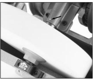
Figure 6. Oil Feeder check ball.
